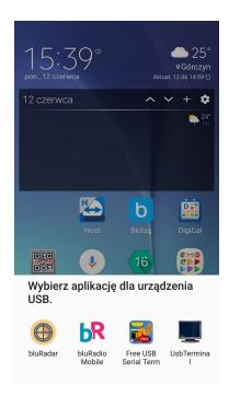
On the main screen of BluRadar you will automatically see a list of all the loggers that are in your proximity, transmitting information to the hub. You must keep in mind that the signal from the logger is transmitted only at the moment of measurement. So, if the measurement interval is set to 15 minutes, the maximum time after which you should see the logger in the app is 15 minutes.
