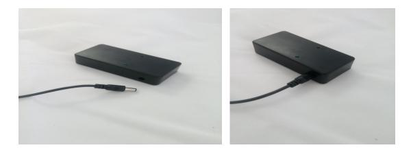
For the best results, repeater should be positioned in proximity of the signal damping element, in a vertical position (diodes located at the bottom), and at least 40cm from the sealing. Repeater shouldn't be installed on the metal surfaces or in proximity of the computers.
