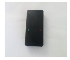
Green diode on repeater means that the device is working.
