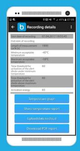
By pressing the "Recording details" button, you will be taken to the page where you can press the corresponding button, you can check the temperature graph, share thetemperature report, upload the data to the cloud and download the report to your phone.
