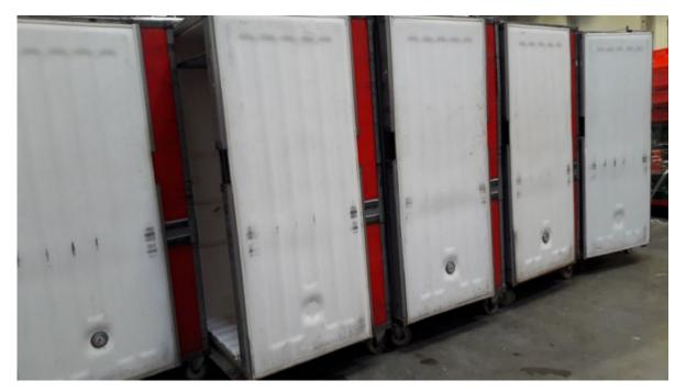
The temperature sensor is integrated in the door at the bottom. This solution of temperature monitoring is susceptible to have mechanical damage and indicates the temperature at the bottom of the container. The expected solution should meet the EN12830 standard.
