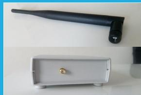
Next, install the antenna, by screwing it into the socket you can find on the back panel of the hub.
