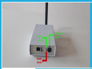
In the presented picture you can see three diodes located on the hub: two green ones (one POWER diode located above the socket and one RF diode) and one ERR red diode. All three diodes should turn on at the moment of connecting the hub and then the red diode should switch off once the hub is connected to the Internet. Below you will find a brief description of each diode and a helpful table with eventual anomalies/issues, their causes and possible solutions.
