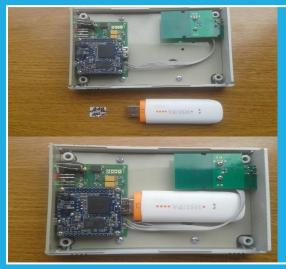
If you are using 2G/3G connection, please open the hub, by unscrewing 4 screws by using a screwdriver. Insert your sim card into a modem, and plug it in into a USB socket as shown on the below pictures. When your modem will be installed, please close the hub by re-fitting the 4 screws.
