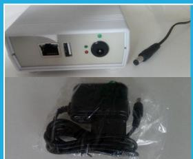
Last step is to connect your hub to the power source, either 230VDC wall socket or via 12V / 24V cigar socket in truck (appropriate adapters are provided with your hub).
