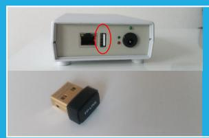
If you have a Wi-Fi option, please plug the module into USB socket located on the front panel of your bub.
